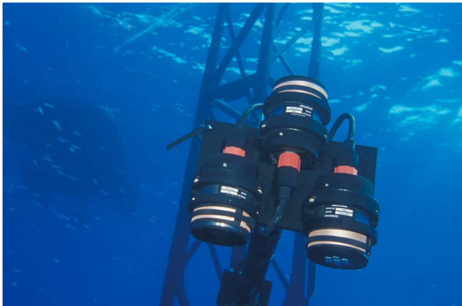
Fig 1. Buoy rads are equipped with copper sheets near detectors, to prevent bio-fouling contamination.
